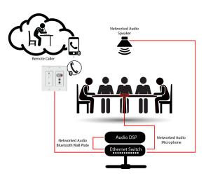
This application diagram highlights the general system connectivity for a networked audio conferencing system utilizing Bluetooth call bridging with Attero Tech's call bridging enabled networked audio products.
