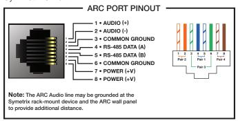
Port Settings: 38.4 kbaud, 8 data bits, 1 stop bit, no parity, no flow control.
